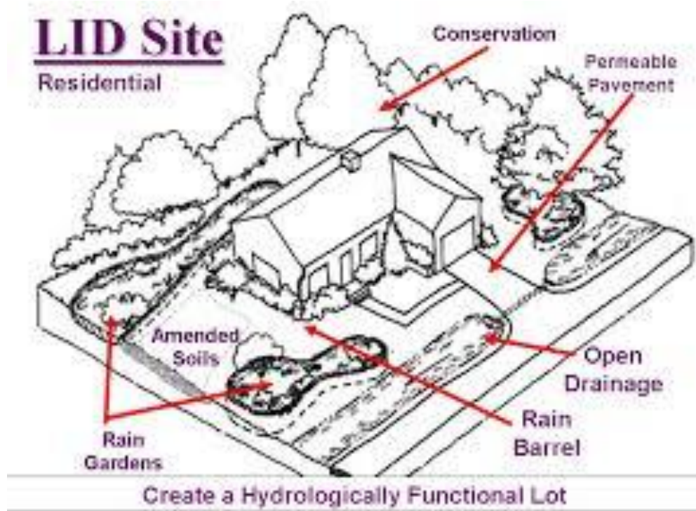
Figure 15: Conceptualized drawing of an urban lot designed to minimize runoff from the site. Future growth plans for the City of Salinas call for 'Low Impact Development' (LID) techniques such as these to reduce stress on the already 'maxed out' Rec Ditch system that would be anticipated as the urban 'impermeable' footprint contributing runoff to the watershed is increased.
