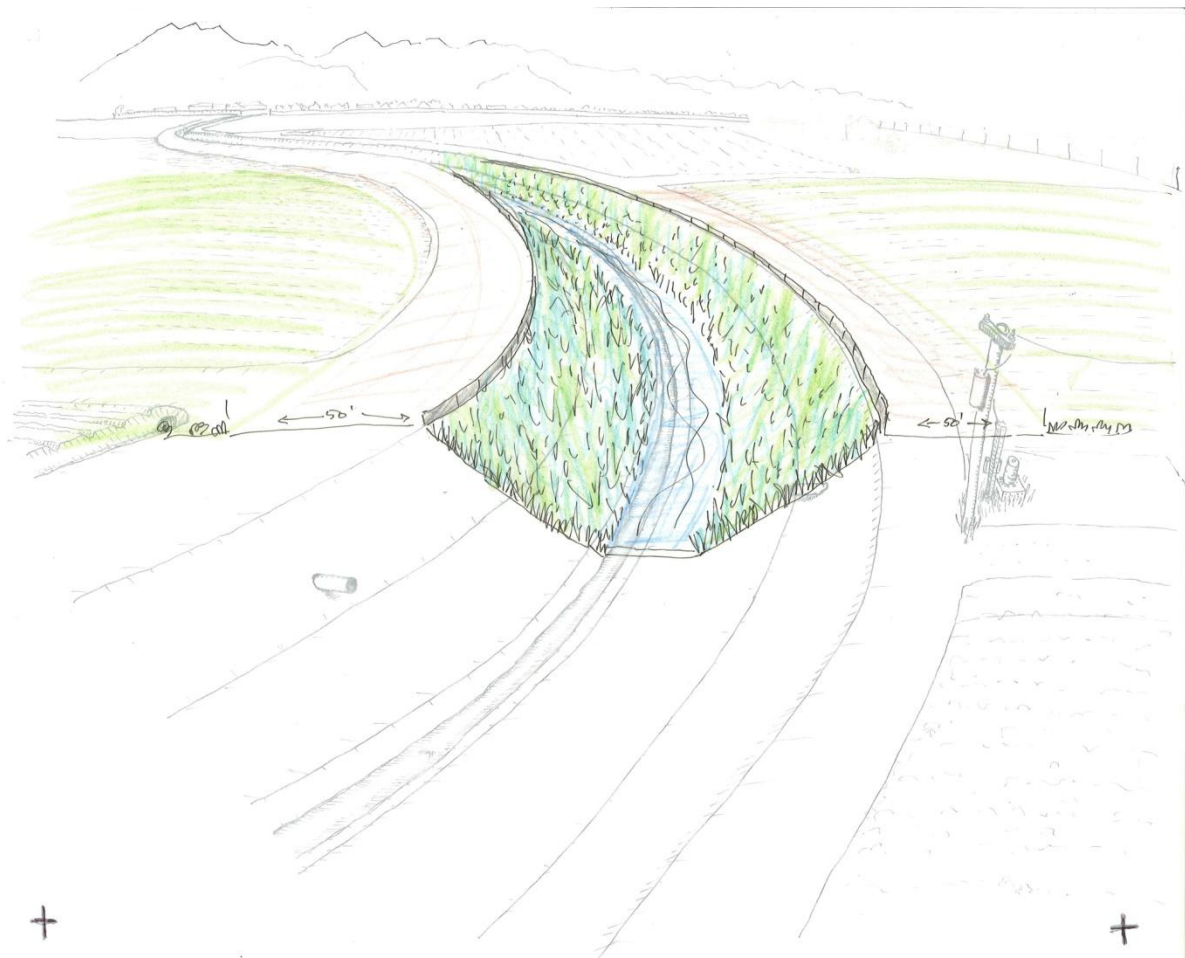
Figure 24: An overlay of the ditch schematic more illustrative of a typical Rec Ditch cross-section with 'bank-to-bank' herbaceous vegetation, calling out specific elements needed to meet food safety concerns: low-stature fence and 50' bare-earth buffers between edge of vegetation and field.
