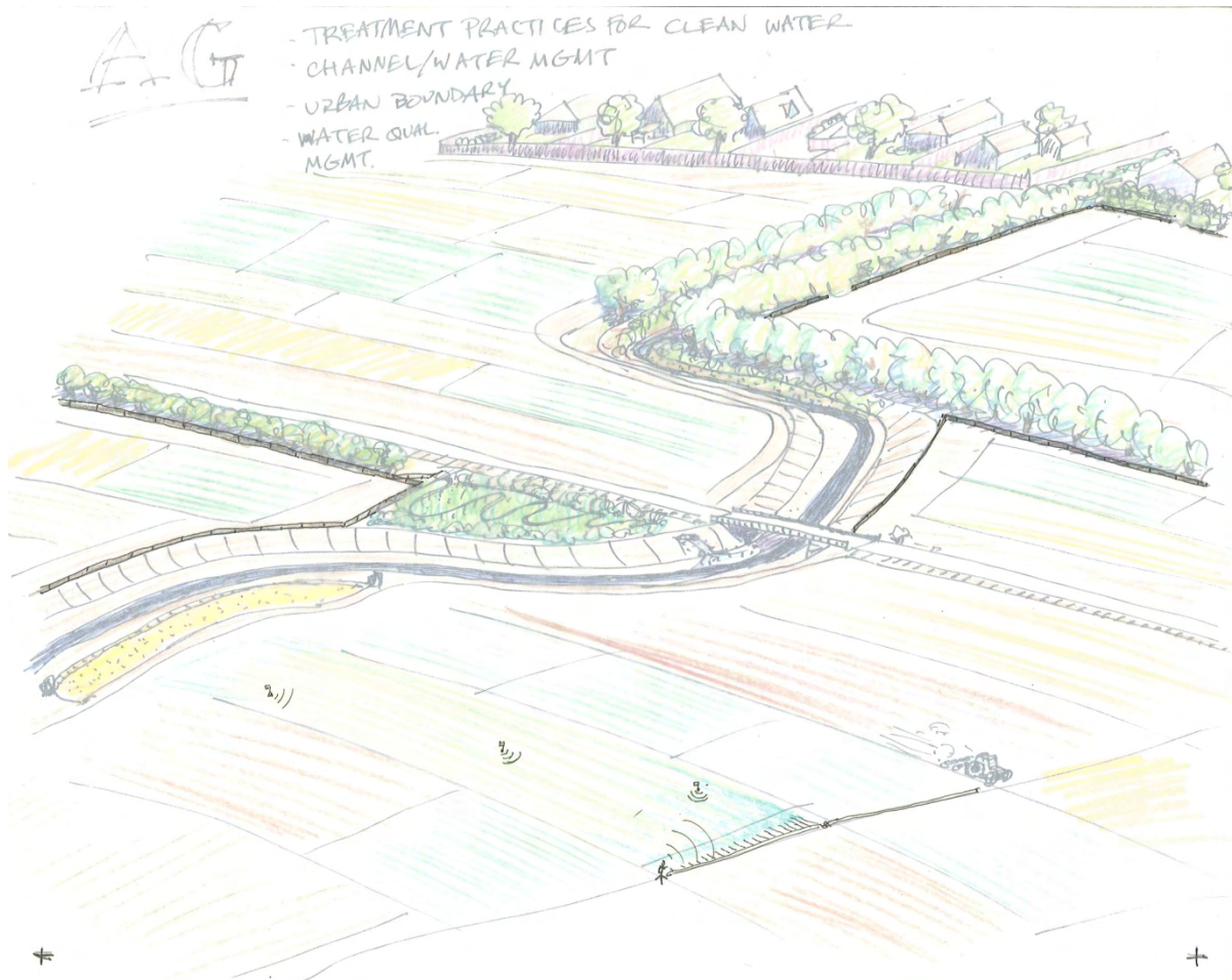
Figure 23: A modification of Figure 3 incorporating comments from interviewees regarding additional farmland practices for water conservation and food safety protection: in-field soil moisture monitoring stations and low-stature “food safety” fences along waterway and pond edges to minimize small wildlife incursion into vegetable production fields.
